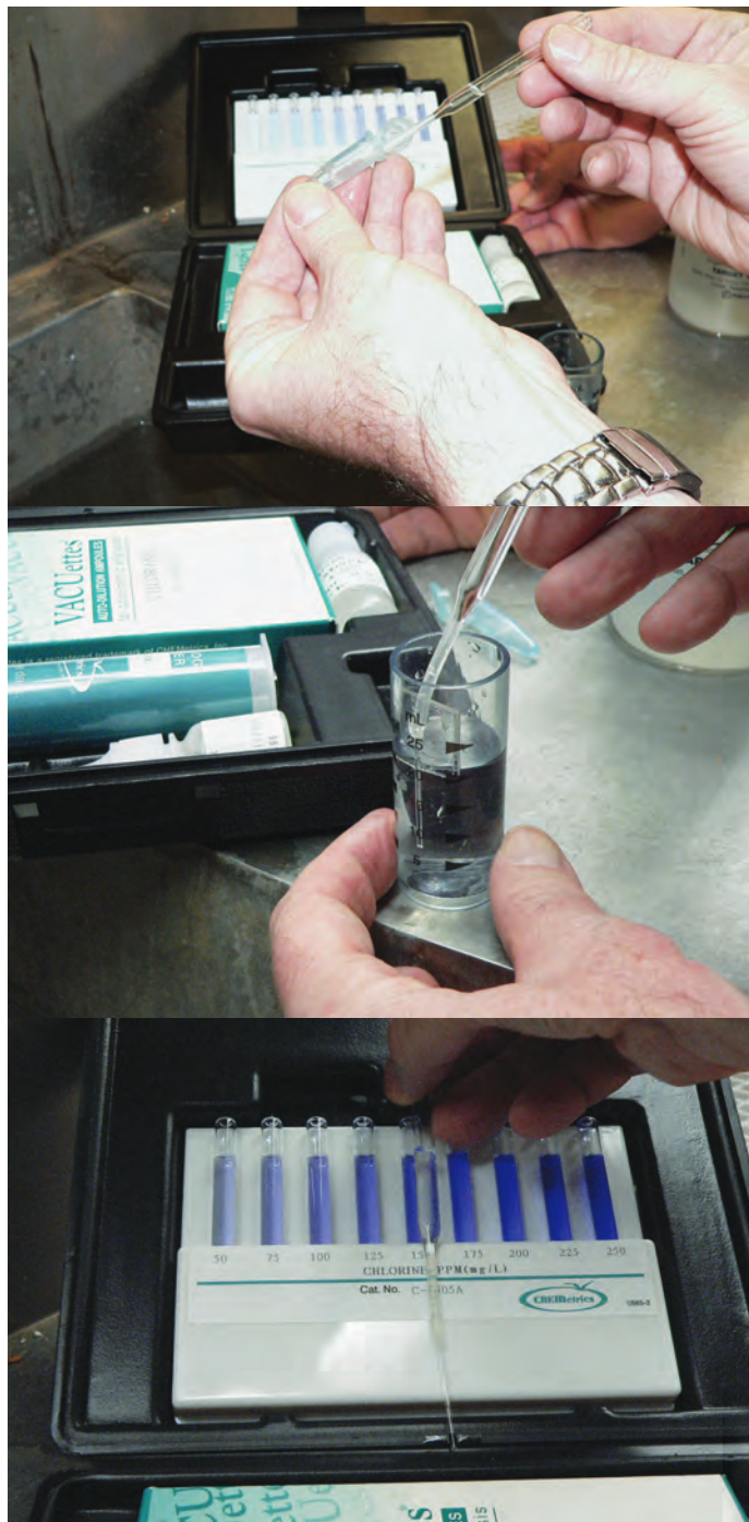
Monitoring dump tank water chlorine levels manually
